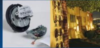
Remote Disconnect Switch Interbase (DSI) option on TWACS ®
